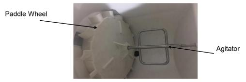
2. Pull on the hand-removable agitator until it is clear of the agitator bushing.
