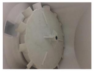
4. Slide the paddle wheel from the motor shaft and remove.
