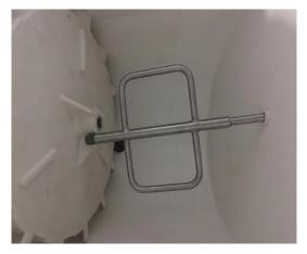
3. Push the agitator toward the back of the bin until the agitator is free of the paddle wheel hub. Remove the agitator by sliding to one side as you pull forward until the agitator shaft clears the bushing.
