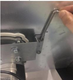
4. Pull the disassembly pin up.
