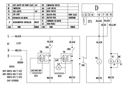
Note: the part in dotted line box is not applicable to some types. Please refer to the real object for the wiring circuit<sub>o</sub>
