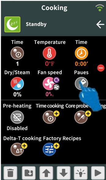
**Noted:** this function is mainly used when the user has set up several cooking phases, when a cooking phase finishes, the user will be reminded to open the oven and take out the food for adding condiments or other processes. After adding condiments or other processes, please put the food into the oven and the cooking process will continue.
